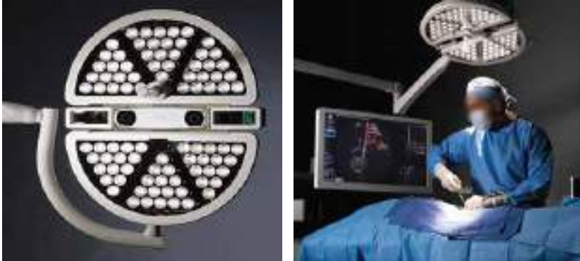
Figure 8: The 7D Surgical System surgical light head contains navigation optics as well as LED lights used for standard lighting 20
